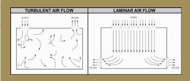
been exhaled. Consider any indoor space and ask the question, "where is the return grille and how many are installed?" In most cases, there is one return grill located in the ceiling, near the thermostat. This is a great location for the thermostat to sense the average temperature of the return air. But what about occupants that are inhaling the off gassing of others in the space? The occupants closest to the return air grille will inhale a higher concentration of airborne particles.
