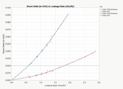
Figure 10. Typical test result from a leakage rate test. A typical mineral fiber tile has a leakage curve (red) and may leak at a rate of about 1.75 [cfm/ft2] at 0.020 [in WC]. The addition of a special soft gasket reduces that leakage rate to about 0.60 [cfm/ft2].
