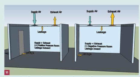
Figure 11. Left, airflow supply into room is greater than exhaust flow, creates "positive pressure room" relative to surroundings, controlled leakage is out of the room. Right, airflow supply into room is less than exhaust flow, creates "negative pressure room" relative to surroundings, controlled leakage is into the room.
