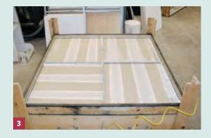
If the sample is a grid and tile assembly, then airflow is normalized by the area of the assembly. If the sample is a single item, such as a fire sprinkler, lay-in light fixture, high hat light fixture or other penetration, the sample tray is sealed so that all air must pass through/around the item under test (Figs. 4, 5, 6, 7, 8, 9). Leakage rate [cfm/ft2] is determined across pressure differences ranging from 0.000 to 0.090 [in WC].
