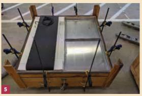
Figure 5. Leak test of a grid installed air cleaner.
