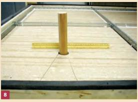
Figure 8. Simulated penetration of a fire sprinkler pipe.
