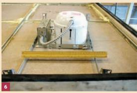
Figure 6. Leak test on a high hat light fixture.
