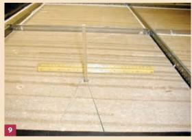
Figure 9. Simulated penetration of a cable tray drop rod.
