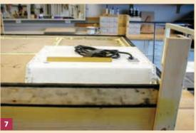
Figure 7. Leak test on a 2x2 [ft] lay-in troffer light fixture.
