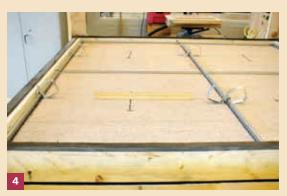
Figure 4. Typical suspended ceiling tiles in test frame.
