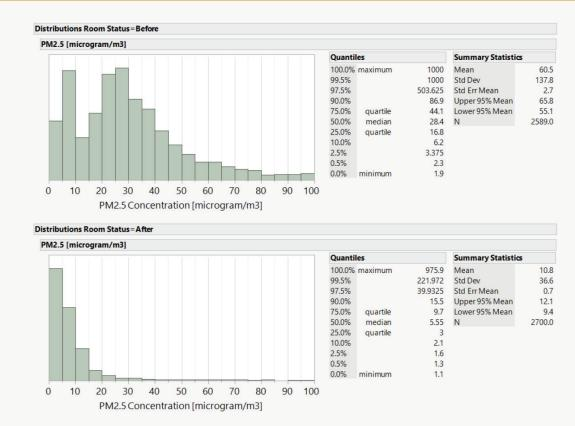
Figure 17. Top chart: PM2.5 concentration before the room was pressurized ranged from 6 to 87 [micrograms/m3]. After the room was pressurized, the PM2.5 count reduced to 2 to 16 [micrograms/m3].
