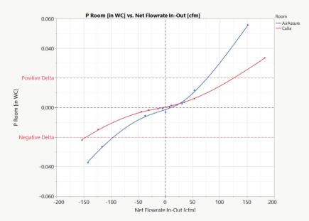
Figure 12. Room pressurization with varying net airflow rates into the room. AirAssure ceilings reduce fugitive leakage, allowing you to achieve a design pressure difference with less net airflow and fan energy. Note that these results are specific to the test room size and the background leakage rate of the enclosure.
