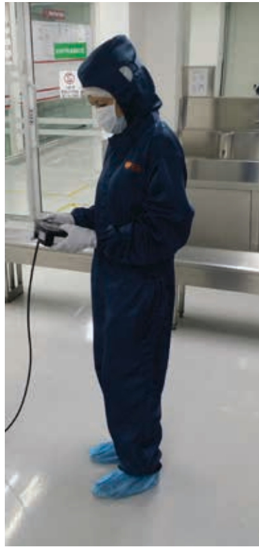
This series of pictures were taken while Yong was doing Cleanroom Performance Testing at a leading pharmaceutical factory. The main production area is under Grade D classification. Occupancy Mode is under at rest condition. From left to right, Picture 1: Yong checking airflow volume from the diffuser by using TSI Alnor Flowhood. Picture 2: Yong on a completed job that required taking the room pressure using TSI Balometer. Picture 3: Yong conducting an airborne particle count test using Lighthouse Solair counter.
