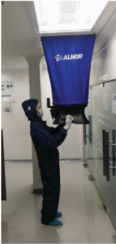
This series of pictures were taken while Yong was doing Cleanroom Performance Testing at a leading pharmaceutical factory. The main production area is under Grade D classification. Occupancy Mode is under at rest condition. From left to right, Picture 1: Yong checking airflow volume from the diffuser by using TSI Alnor Flowhood. Picture 2: Yong on a completed job that required taking the room pressure using TSI Balometer. Picture 3: Yong conducting an airborne particle count test using Lighthouse Solair counter.
