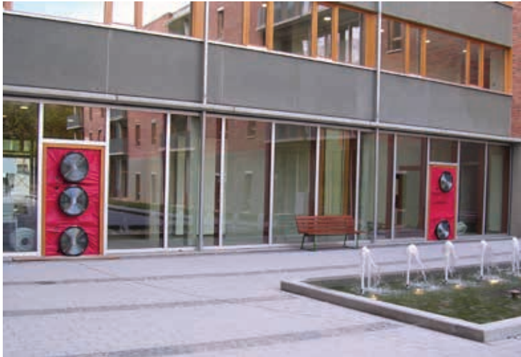
Building enclosure test using two Minneapolis Blower Doors.
