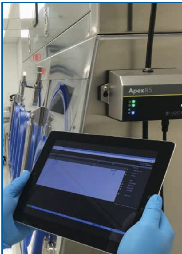
Fig.2 Cleanroom operator connecting to EMS monitoring particle counts inside an isolator
