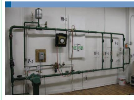
The Bledsoes established a hands-on test lab for test and balance training for industry supervisors and technicians. This picture shows water pipes and ductwork in the test lab.
