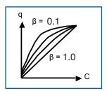
A high value of valve authority means that the differential pressure is close to constant and the relationship between Cv value and water flow becomes quite linear. A low value, on the other hand, means that the differential pressure will increase a lot when the valve closes, resulting in large nonlinearity between Cv value and flow. The lower the valve authority is, the more nonlinear the curve becomes.
